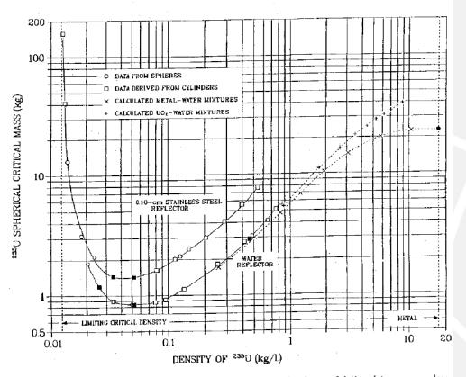
Fig. 10. Critical masses of homogeneous water-moderated U(93.2) spheres. Solution data appear unless indicated otherwise.
