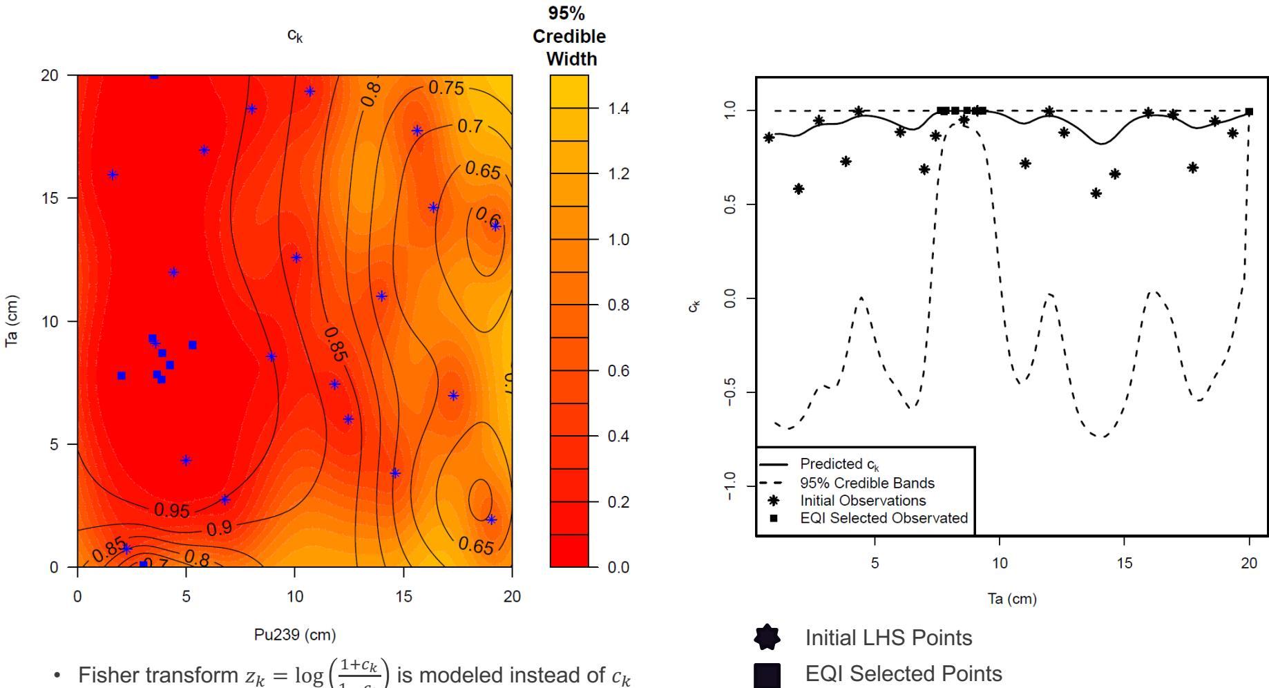
Optimized configuration (4.25 cm  $^{239}\text{Pu}$  surrounded by 8.24 cm Ta) for aliquot casting yielded  $c_k$  of 0.9997.
