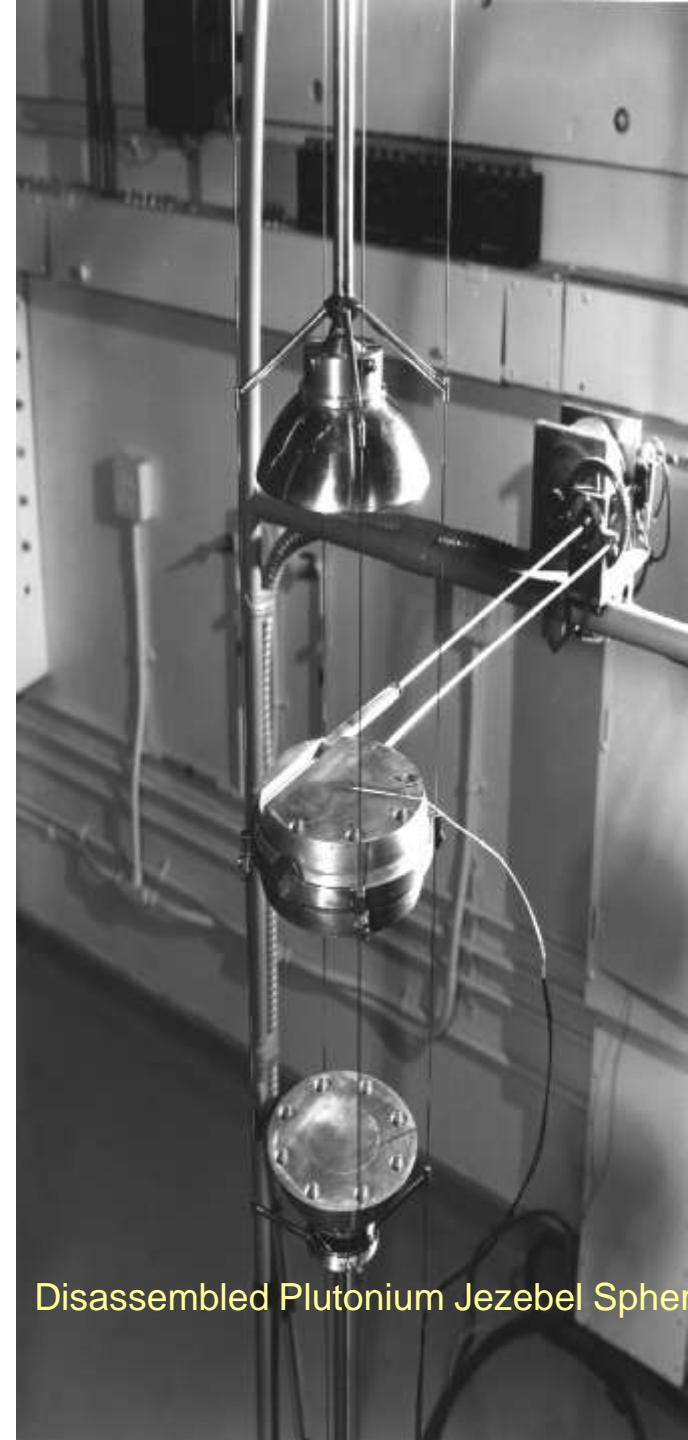
Disassembled Plutonium Jezebel Sphere
