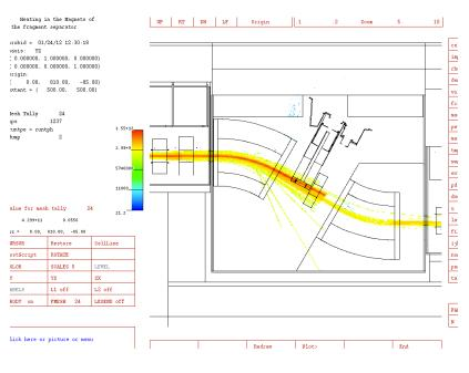
Primary ion beam as it collides with the beam dump
