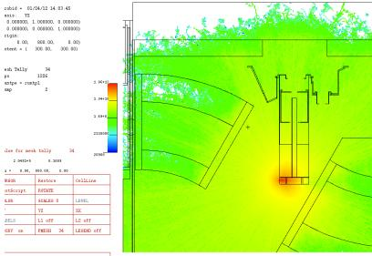
**Neutron field** produced by ion beam collisions with target
