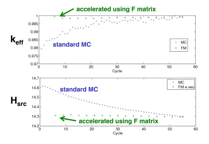
Acceleration using fission matrix for 3D full-core reactor benchmark
