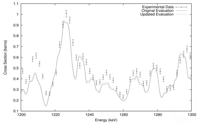
Inelastic cross section of <sup>56</sup>Fe before ( $\chi^2$  = 23.6023) and after ( $\chi^2$  = 22.9036) the adjustment based on integral experimental data plotted on top of differential experimental data of Perey, presented with one standard deviation error bars.
