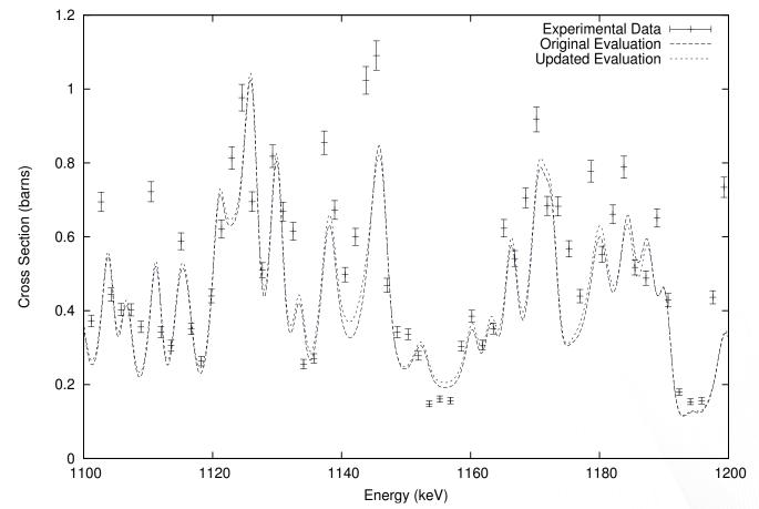
Inelastic cross section of <sup>56</sup>Fe before ( $\chi^2$  = 73.3382) and after ( $\chi^2$  = 73.6877) the adjustment based on integral experimental data plotted on top of differential experimental data of Plompen, presented with one standard deviation error bars.
