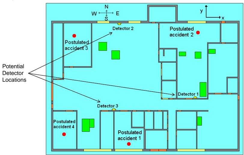
2 d) Calculate neutron and gamma doses for each detector location:
