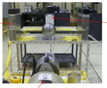
SNAP detector: Single He-3 tube inside polyethylene and Cd. Has a removable 1 inch-thick poly shield.
