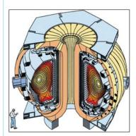
Schematic of DIII-D Tokamak National Fusion Research Facility
