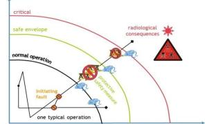
→ Strict limits on <u>"operating" parameters</u>, to ensure the control of the nuclear criticality risks in these facilities.
