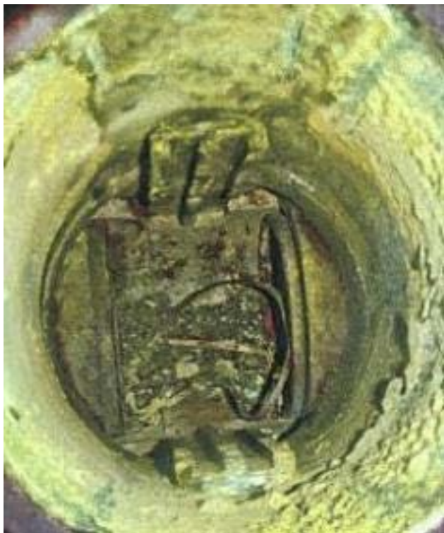
Inside of a 12" G-17 Valve Body with a Uranyl Fluoride (UO 2 F 2 ) coating
